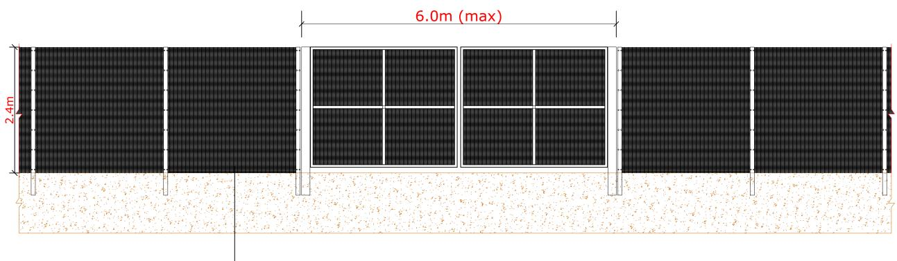
Welded steel wire mesh (SR2) —
